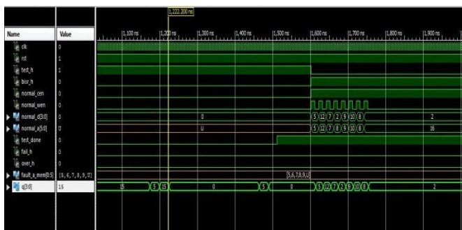
Fig.5: Simulation Wave Forms of BISR Module
